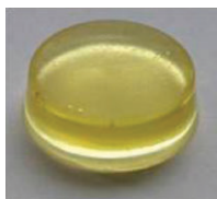
Fig. 1 Pd-doped iongel pellet.
